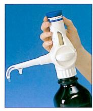
TO SET the volume, rotate the graduated ring to the required position. Once selected the set volume is automatically locked in position, preventing accidental adjustment.
